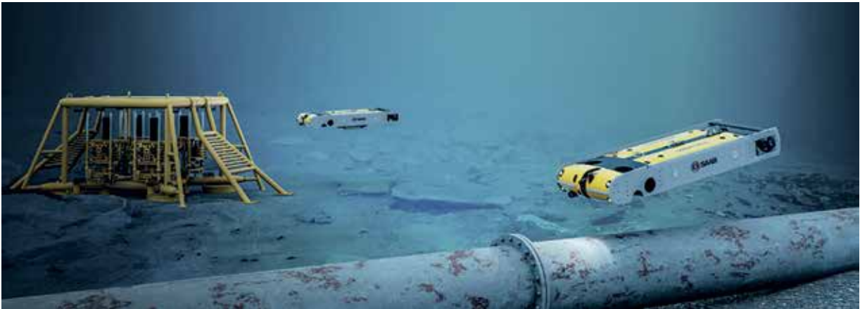
Repair drone for underwater infrastructure, Saab Sabertooth (source: SAAB)
