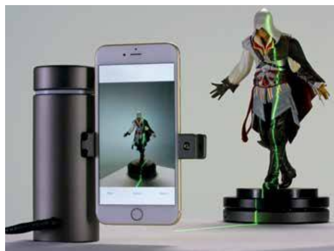
3D-scannen via de smartphone. ( https://eora3d.com )
